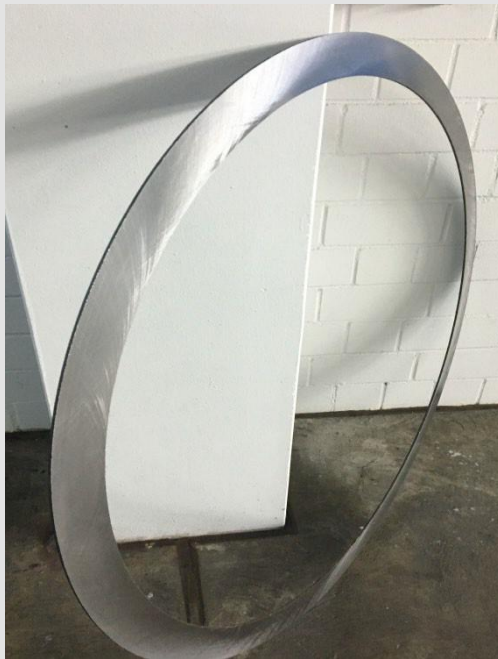
Austenitic stainless steel X2CrNiMo17-12-2
